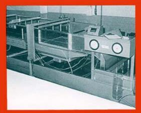
Hydraulic testing of Neenah drainage grotos is now being conducted in this full size flume at our own laboratory. Write for our free report
