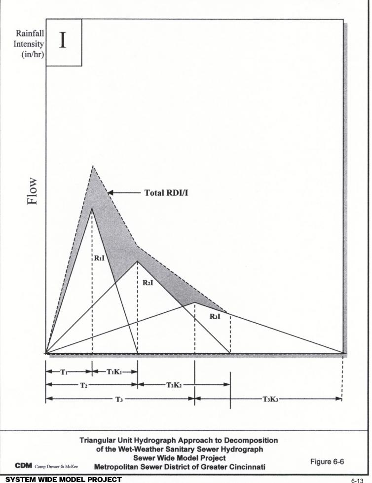
5. Finally, the project team will verify the R, T, and K parameters by using them along with catchment areas to develop inflow hydrographs for a more complex rainfall event. These hydrographs are then routed through the collection system with the model developed and compared with measured hydrographs for this event.
