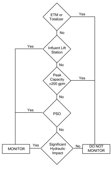
Figure 8-1 Pump Station Flow Monitoring Decision Flow Chart
