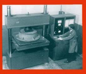
To determine load bearing qualities of Neenah castings, pressitests are conducted as part of our research program. Write for our wheel load capacities monual.
