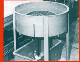
Test tank in which over 2000 separate inflow tests were conducted to develop data for this report.
