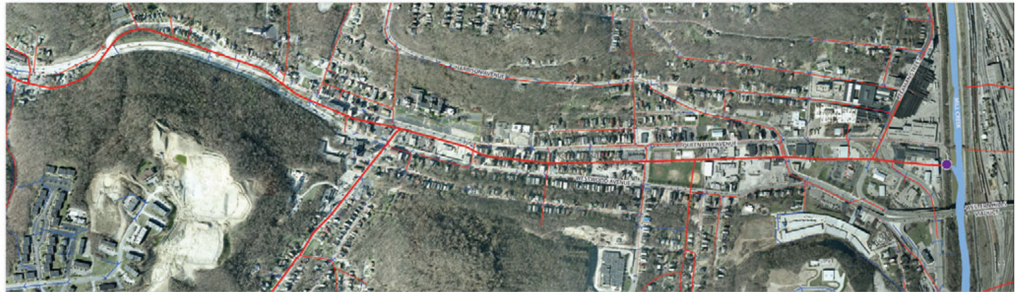
Lick Run Corridor: Existing Conditions Currently, the Lick Run stream runs through an underground 19.5-foot diameter combined sewer. ● Combined Sewer Overflow (CSO) — Existing Combined Sewer — Mill Creek
