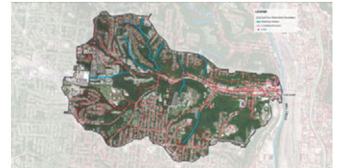
Existing stream network. Currently, the Lick Run stream runs through an underground 19.5-foot diameter combined sewer.
