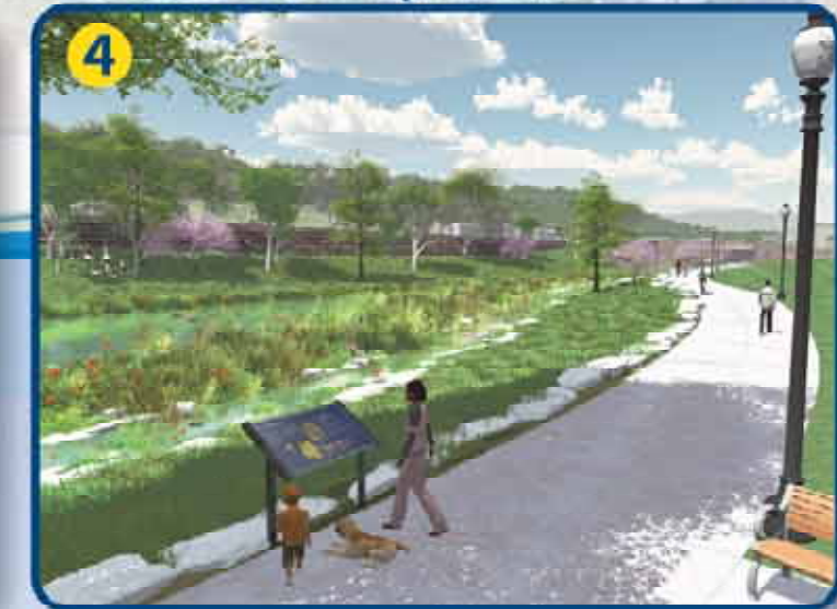
(Looking South toward Westwood) This image depicts the character of the proposed urban waterway at the water quality feature. The multi-purpose path provides safe, well-lit access. During low volume rain events, runoff flows north of the water quality feature to Mill Creek. During high volume rain events, water flows both north of and into the water quality feature. This feature provides valuable terrestrial and aquatic habitat.
